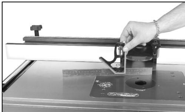
2. Use a straightedge to test the plate for level with the table top.
